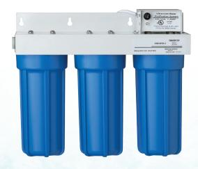
**Aqua Flo Product's patented UVB Series** is designed to provide disinfected water at a flow rate of 2 gallons per minute. In addition to disinfection, water is filtered through our 0.5 micron Extended Pass Carbon Block (EPCB) filter. Our double and triple models provide you with additional filtration with sediment and activated carbon filters.
