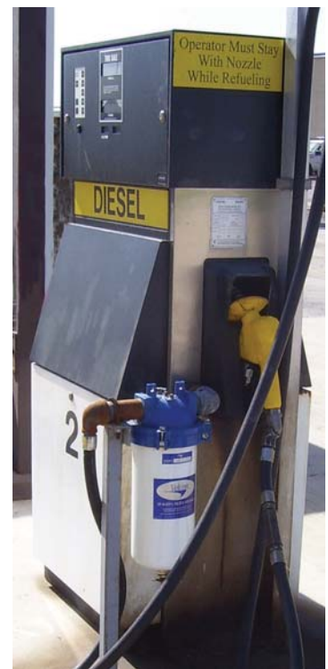
VF-61 connected to a diesel fuel dispenser
